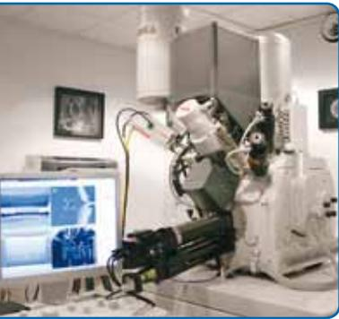
Flagships: FEI Nova NanoLab 200 DualBeam FIB and the FEI Helios NanoLab DualBeam FIB
