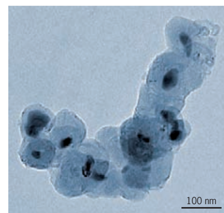
TEM image of carbon nano-onions with encapsulated catalyst particles.
