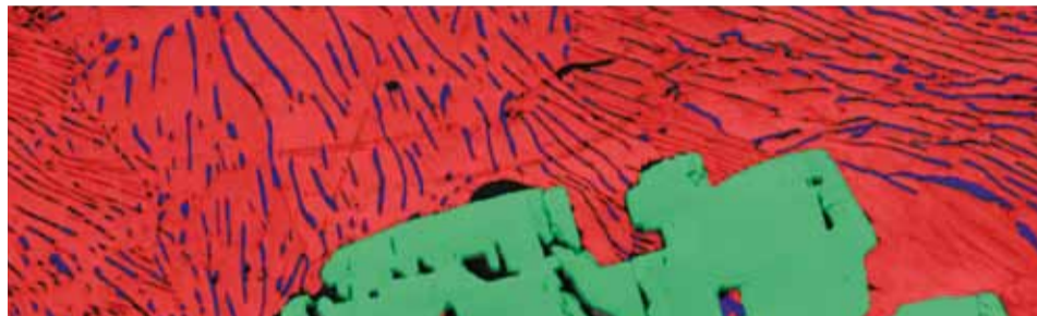
Orientation map (top) and phase map (bottom) of a slag sample collected with EBSD. Large TiN grains (lower part of maps) are in a matrix of ferritic iron and cementite.
