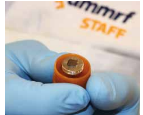
One of the standards to be used in the calibration of a scanning electron microscope.
