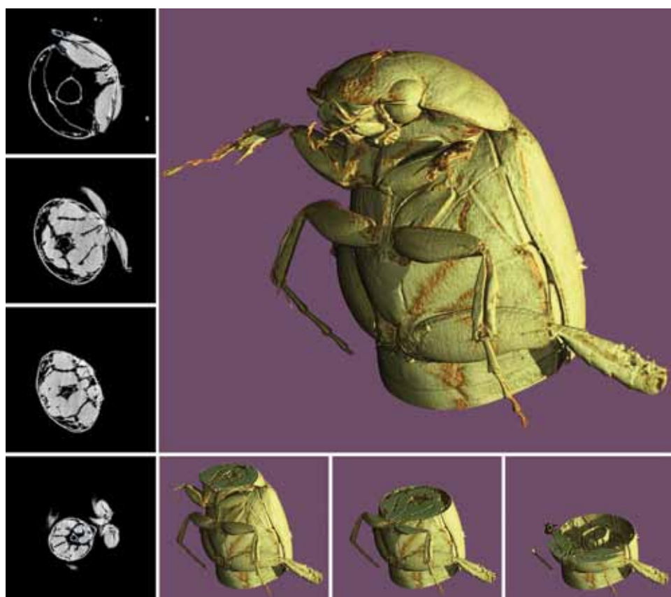
Right: 3-D reconstruction of a christmas beetle from 3.2 GB of X-ray microtomography data (beetle is approx. 10 mm in length). Left: four greyscale images from a set of over 1000. Data-MINX will support transfer, searching and storage of such large data sets such as these.
